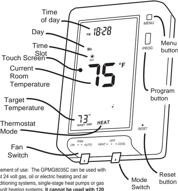
Statement of use: The GPM8035C can be used with most 24 volt gas, oil or electric heating and air conditioning systems, single-stage heat pumps or gas millivolt heating systems. It cannot be used with 120 volt heating systems or multistage heat pumps.
